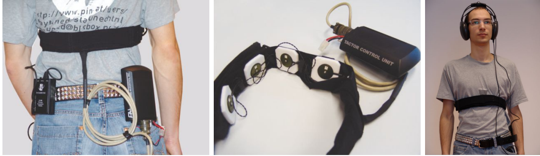
Figure 5.2: The waist-belt system consisting of the vibro-tactile belt, the InterSense transceiver, and the belt controller; a detailed view of the waist belt and the Tactor Control Unit; the author wearing the belt and the headphones during an experiment (from left to right).
