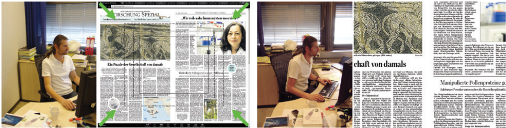
Figure 4. The mat attached to the backrest (y-axis only) is used for controlling the “zoom level” of the screen content. When sitting upright (left-hand side), the content is shown in original size (100%), the more leaning forward (right-hand side), the higher the magnification of the screen content.
