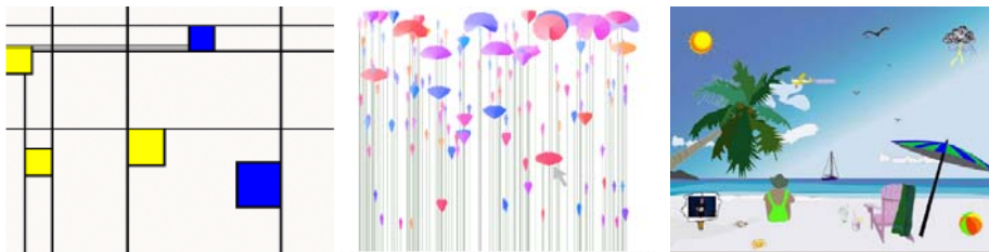
Fig. 2. Informative Art [18] ( left ), inspired by Mondrian, in real time shows the expected weather situation or urban bus traffic situation; PeopleGarden [20] shows user activities in terms of message densities from posting onto a message board ( center ); InfoCanvas [16] ( right ) displays multiple sources of information ranging from NASDAQ Composite Index to the number of employees present at work in real time in a beach scene.
