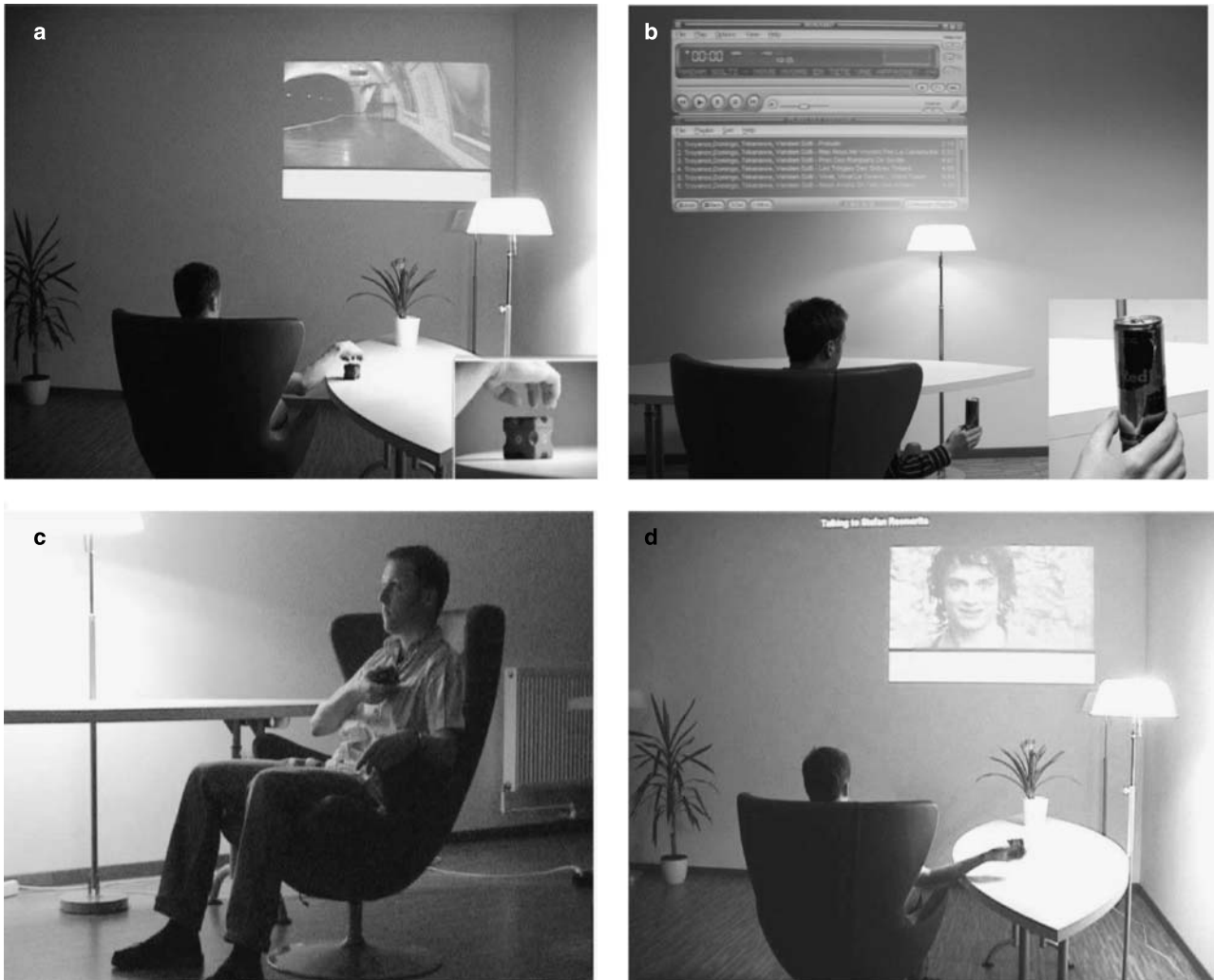
Fig. 8. Application snapshots. (a) TV control with chair and cube, (b) Music player control with cylinder, (c) Accept a phone call, (d) Terminate the call
