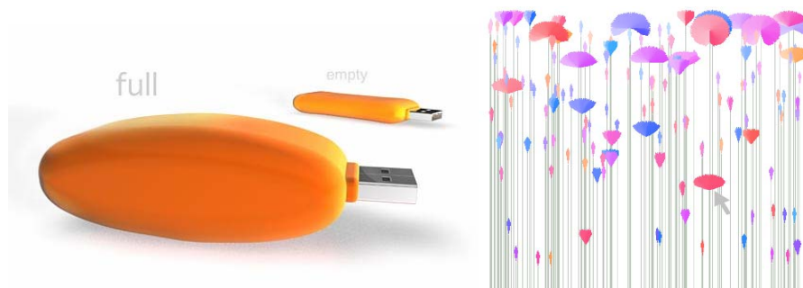
Fig. 1. A physical object (memory stick) designed for the purpose of being an ambient display – it intuitively displays the amount of used storage by the shrinking and growing size of the object (Flashbag: http://www.plusminus.ru/flashbag.html , left). The People Garden [33] figural Informative Art design shows user activities in terms of message densities from posting onto a message board ( right ).
