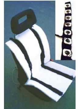
Seat with 2x8 vibro-tactile elements (used for simulation and in real studies)
